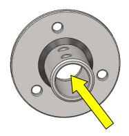
8. Unscrew the mounting bracket from the tube on the wiring end. Place it back in the marked mounting location and mark a point in the centre.Drill a 6mm or larger hole at the centre for wiring.
