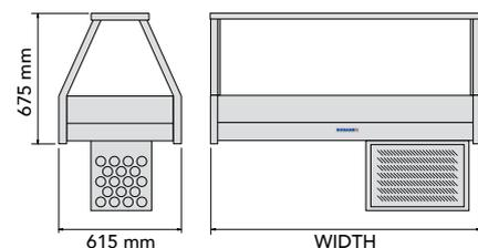
Note: For ERX model range overall height dimensions, add height of motor cage (450 mm).
