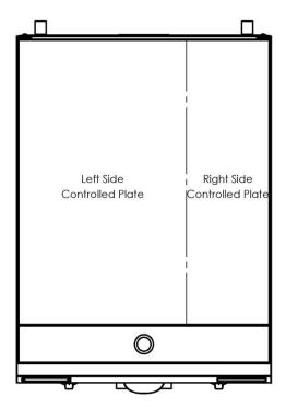
The hotplate is designed in such a way that heat pools in the centre of the hotplate, with the front and rear corners being comparatively cooler. This allows the user to balance the cooking times of multiple products/foods that require different temperatures or times to cook.
