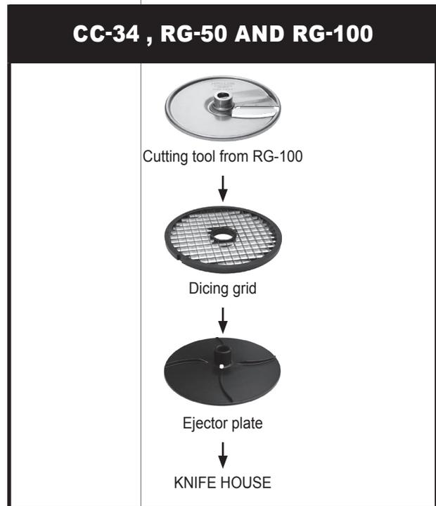
**WHEN USING SLICER, CRIMPING SLICER
